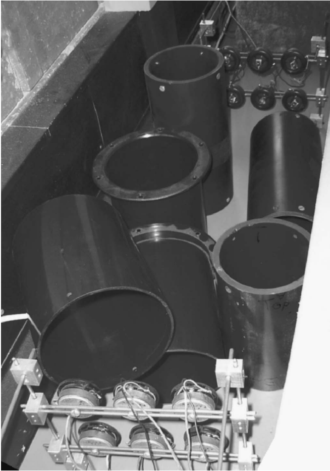
FIG. 4. Photograph of the experimental rig used to obtain the impulse response functions showing transmitter and receiver arrays and randomly oriented objects used to emulate a difficult environment through which to transmit.
