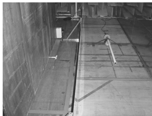
FIG. 9. The experimental setup for measurements in an anechoic chamber for a parallel barrier placed in front of a façade surface. The setup for a street canyon is not shown in the diagram.
