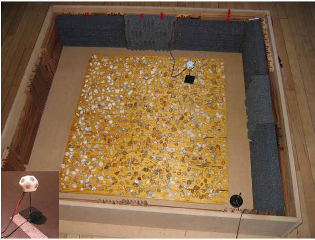
FIG. 6. (Color online). Photograph of the flat room scale model showing the speaker, microphone, QRDs, foam, and rocks. A detailed photo of the scale-model sound source is shown in the left corner.
